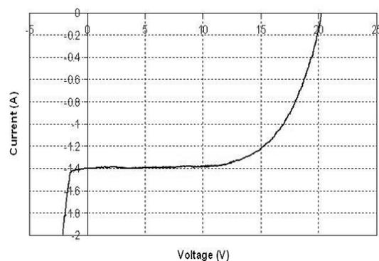
**FIGURE 6.** A typical IV-curve of a 30 cell sub-module operating at around 14 suns optical concentration.
