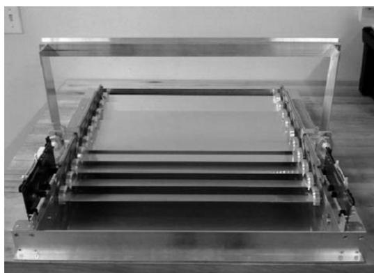
**FIGURE 5.** The test rig developed by Chromasun using representative mirror sections and full tracking capability.
