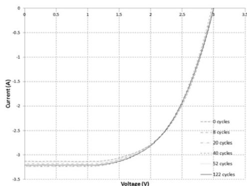
**FIGURE 4.** I-V curves during hot thermal cycling, showing no significant changes in the electrical performance.
