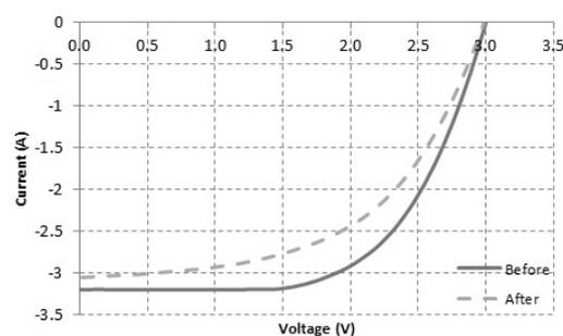
**FIGURE 3.** I-V curves of one of the initial prototypes before and after the thermal cycling test.
