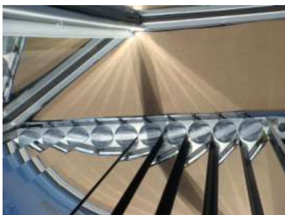
Figure 2: Detail of ganged reflectors in the prototype MCT, showing focal performance at the end-plane.
